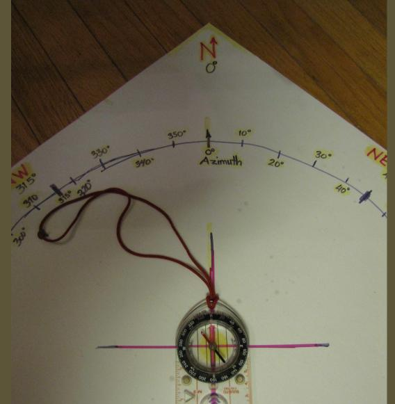
6. Lay the magnetic compass on the mat so the center is on the center of the map and it points to the North. The marks on the compass should line up with the marks on your rose. The Needle may not be lined up at this point.
